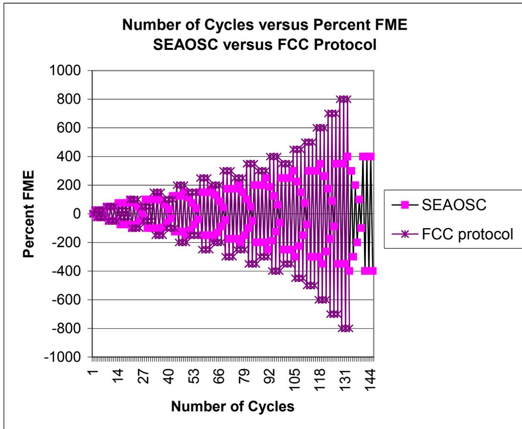
Figure 2.1. Comparison of SEAOSC and FCC loading protocol.
